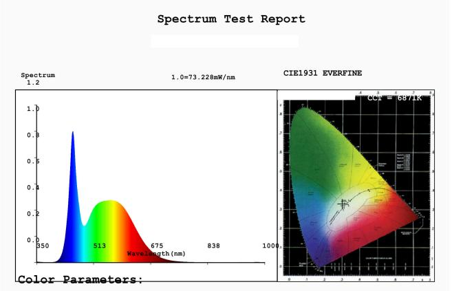
Chromaticity Coordinate:x=0.3069 y=0.3248/u'=0.1953 v'=0.4652 CCT=6871K(Duv=0.0040) Dominant WL:Ld =487.5nm WL:Lc = --nm Purity=9.6% Ratio:R=13.0% G=80.8% B=6.1%;;Peak WL:Lp=453.7nm FWHM=26.3nm Render Index:Ra=83.6 AvgR=76.4 TM30:Rf=83 Rg=93 Lav=535.9nm
